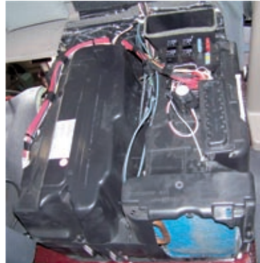
Figure 1 – ParkSmart Unit (shown with cabinet removed)
